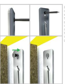
EPDM gasket on screw extends through the plate and compresses against the air barrier to help seal the screw penetration
